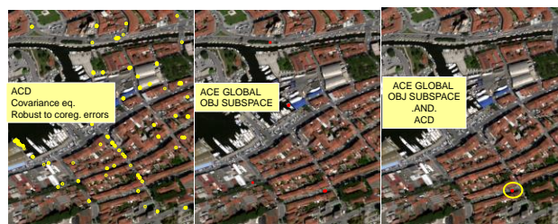
Fig. 1 (a) ACD map, (b) SSB-OR map, (c) combining (“and” operator) ACD and SSB-OR maps one finds the position where the searched object has moved in the test image.
